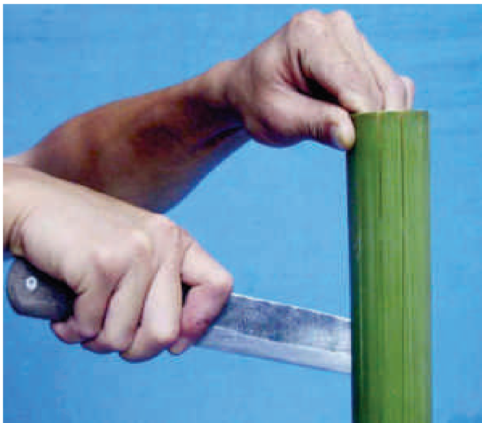
Step 3: Divide the culm into silvers of equal width
