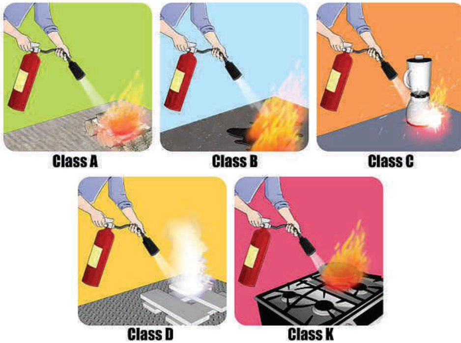
Figure 7.1.2 Classification of Fire Extinguisher
