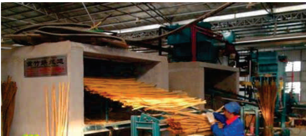
Figure 2.2. 3Drying Bamboo Silver using dryer machine
